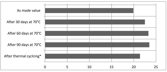
\* Thermal cycling: 25 cycles of 6 hours duration from -30°C to 70°C
